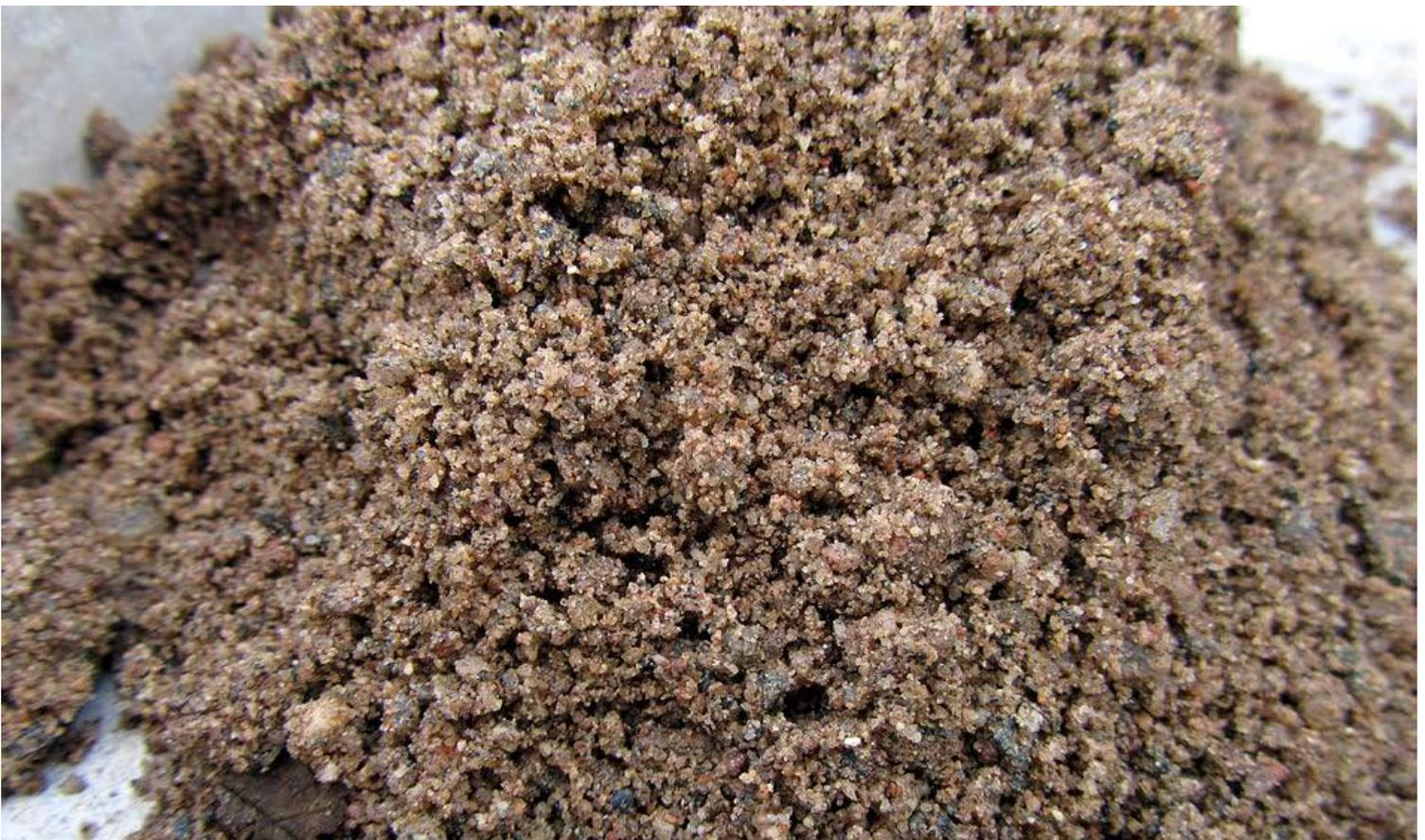
I use **sharp sand** from a builders' supplier or quarry, you can see it has a range of particle size. Not what is called 'builders' sand' the UK; that is too fine and has been graded through a finer screen to remove the larger grains and is used for making a mortar mix with cement to lay bricks.
