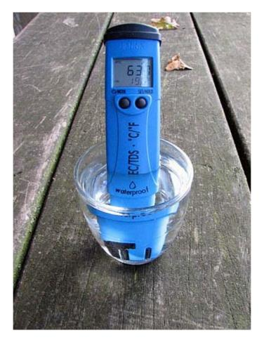
In the cup is tap water straight out of our taps. Notice the reading of 630  $\mu s.$
