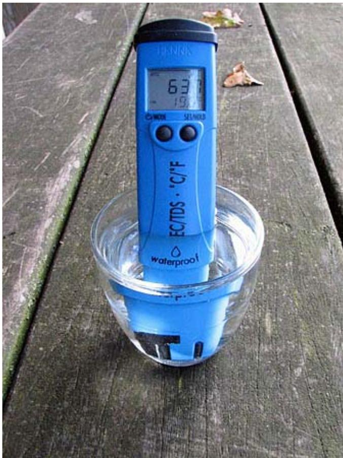
In the cup is tap water straight out of our taps. Notice the reading of 630  $\mu\text{s}$ .
