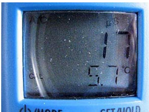
Next we measured a sample of rainwater out of our storage tank, which collects rainwater from the roof of our large polytunnel. This gave a reading of just 17  $\mu\text{s}$ .
